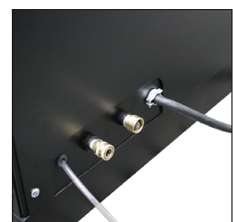
Detergent siphon hose, quick connect and garden hose connections
